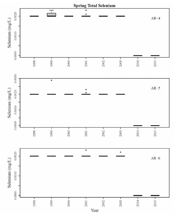
**Figure B.29.** Total selenium concentrations summarized seasonally (April-July) at water quality monitoring sites AR-4, AR-5, and AR-6 on the Upper Arkansas River. The method detection limit (MDL) is indicated by single, horizontal lines.
