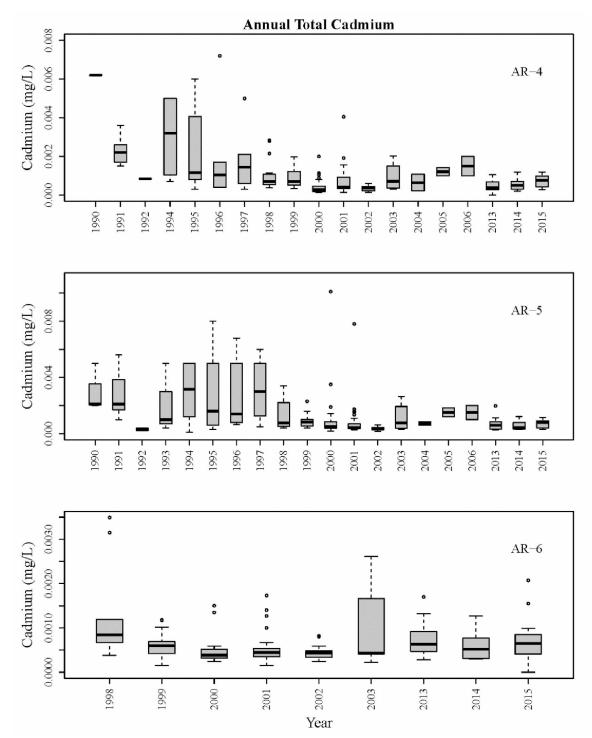
**Figure B.9.** Total cadmium concentrations summarized annually at water quality monitoring sites AR-4, AR-5, and AR-6 on the Upper Arkansas River. The y-axis was limited excluding one observation at AR-4 of 0.014 mg/L in 1995, and one observation at AR-5 of 0.038 mg/L in 1998.
