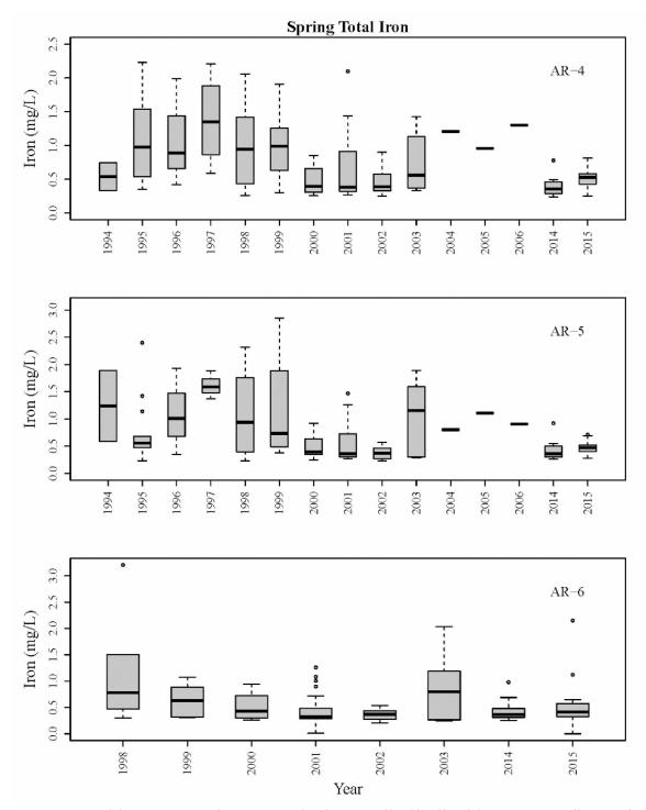
**Figure B.17.** Total iron concentrations summarized seasonally (April-July) at water quality monitoring sites AR-4, AR-5, and AR-6 on the Upper Arkansas River. The y-axis was limited to exclude one observation at AR-4 of 5.849 mg/L in 2001, and two observations at AR-5 of 5.01 mg/L in 1999 and 5.968 mg/L in 2001.
