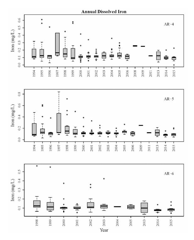
**Figure B.18.** Dissolved iron concentrations summarized annually at water quality monitoring sites AR-4, AR-5, and AR-6 on the Upper Arkansas River. The y-axis was limited to exclude one observation at AR-4 of 1.684 mg/L in 1998, and one observation at AR-5 of 1.24 mg/L in 1999.
