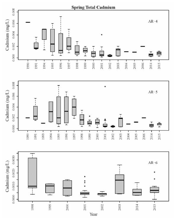
**Figure B.10.** Total cadmium concentrations summarized seasonally (April-July) at water quality monitoring sites AR-4, AR-5, and AR-6 on the Upper Arkansas River. The y-axis was limited to exclude one observation at AR-4 of 0.014 mg/L in 1995, and one observation at AR-5 of 0.038 mg/L in 1998.
