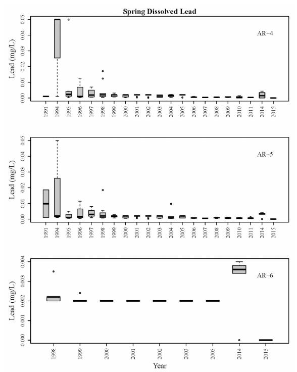
**Figure B.23.** Dissolved lead concentrations summarized seasonally (April-July) at water quality monitoring sites AR-4, AR-5, and AR-6 on the Upper Arkansas River. The method detection limit (MDL) is indicated by single, horizontal lines.
