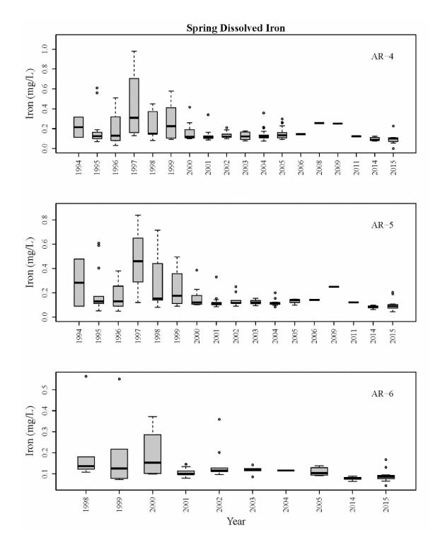
**Figure B.19.** Dissolved iron concentrations summarized seasonally (April-July) at water quality monitoring sites AR-4, AR-5, and AR-6 on the Upper Arkansas River. The y-axis was limited to exclude one observation at AR-4 of 1.684 mg/L in 1998, and one observation at AR-5 of 1.24 mg/L in 1999.
