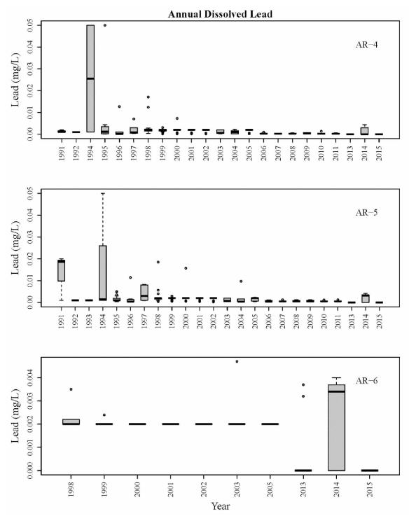
**Figure B.22.** Dissolved lead concentrations summarized annually at water quality monitoring sites AR-4, AR-5, and AR-6 on the Upper Arkansas River. The method detection limit (MDL) is indicated by single, horizontal lines.
