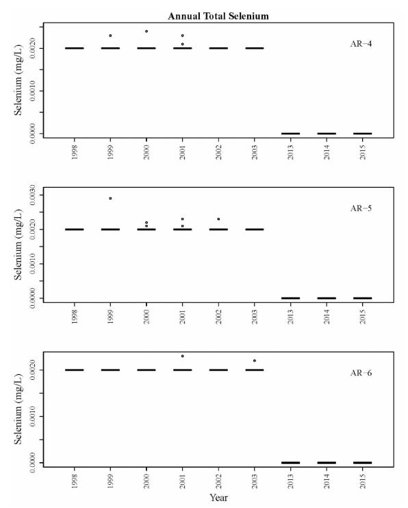
**Figure B.28.** Total selenium concentrations summarized annually at water quality monitoring sites AR-4, AR-5, and AR-6 on the Upper Arkansas River. The y-axis was limited to exclude one observation at AR-4 of 0.011 mg/L in 2003, and one observation at AR-5 of 0.007 mg/L in 2003. The method detection limit (MDL) is indicated by single, horizontal lines.
