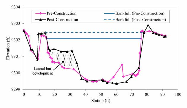
**Figure 8.1.** Comparison of pre- and post-construction morphology and bankfull elevations for treatment cross-section XS-10.
