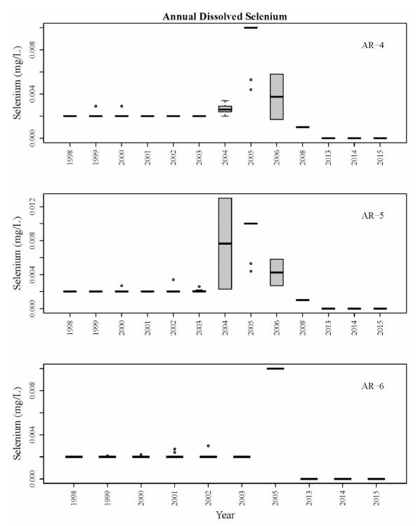
**Figure B.30.** Dissolved selenium concentrations summarized annually at water quality monitoring sites AR-4, AR-5, and AR-6 on the Upper Arkansas River. The y-axis was limited to exclude two observations at AR-4 of 0.035 mg/L in 2005, and observations at AR-5 of 0.035 mg/L in 2005. The method detection limit (MDL) is indicated by single, horizontal lines.
