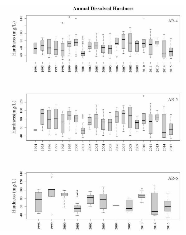
**Figure B.37.** Dissolved water hardness (as mg/L CaCO<sub>3</sub>) summarized annually at water quality monitoring sites AR-4, AR-5, and AR-6 on the Upper Arkansas River.
