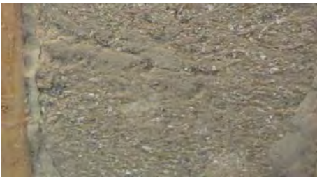
Dense Pack Cellulose: R3.2-R3.8 per inch Cost: $2.00 to $4.00 per sq. ft. installed
