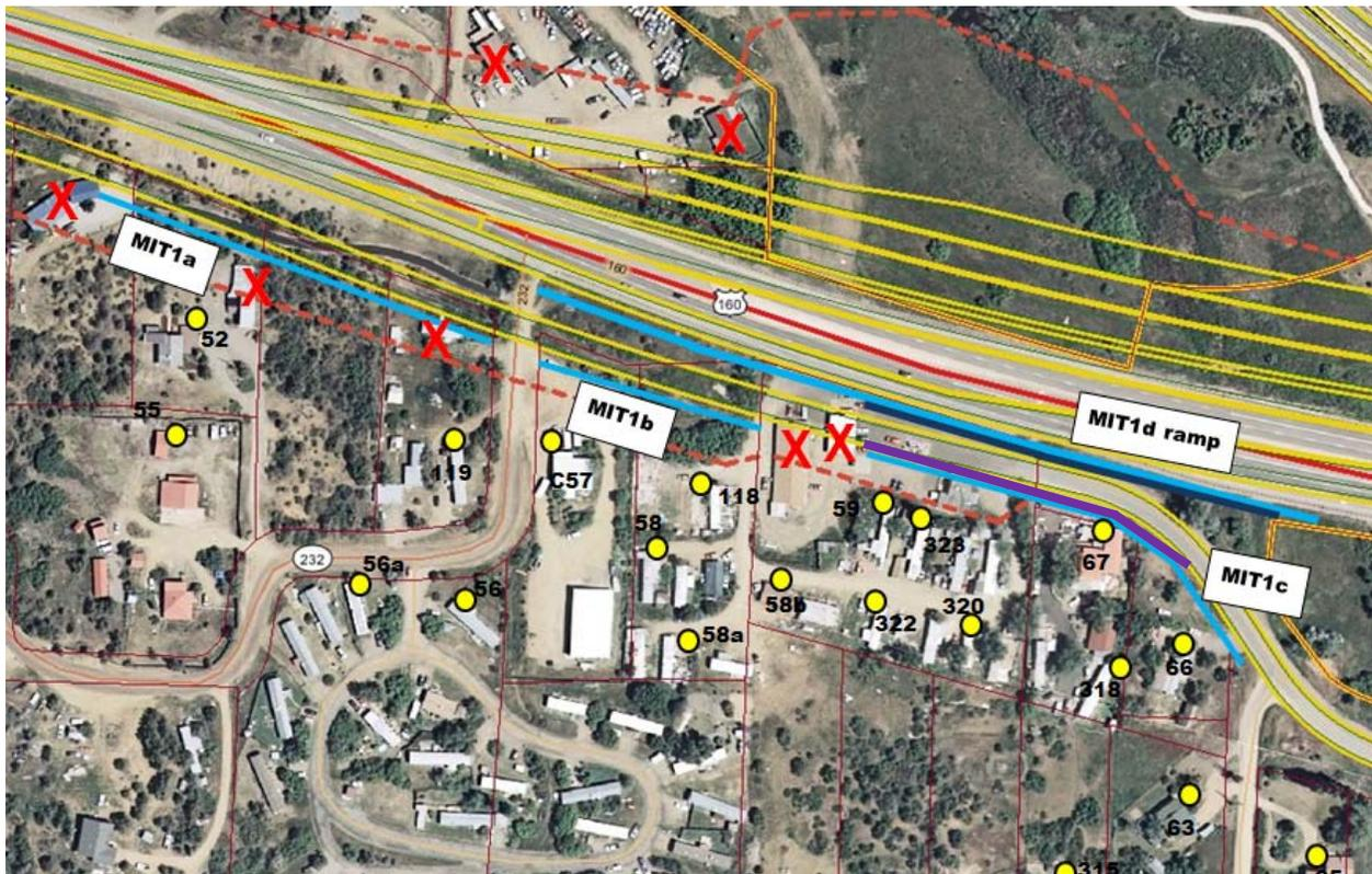
Wall locations were analyzed along the service road for mitigation scenario MIT 1 and included 3 walls, referred to as a, b, and c (MIT 1a,b,c) and along the shoulder of the US 160 to County Road 233 ramp (MIT 1d). Walls MIT 1a-c were sited to allow continued roadway access at County Road 232 and at a consolidated driveway access near R59.
