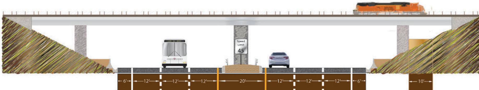
Figure 3-9. Potential Reduced-Width, Six-Lane Urban BNSF Railroad Crossing
