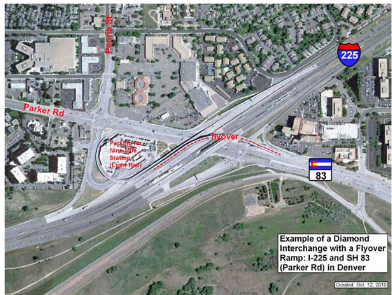
Figure 2-13. Aerial Photo of a Diamond Interchange with Flyover Ramp at I-225 and SH 83 in Denver
