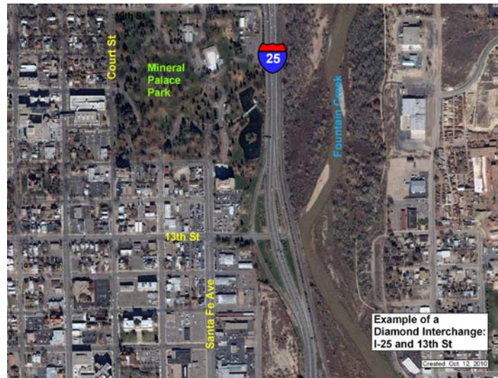
Figure 2-12. Aerial Photo of the Diamond Interchange at I-25 and 13th St. in Pueblo
