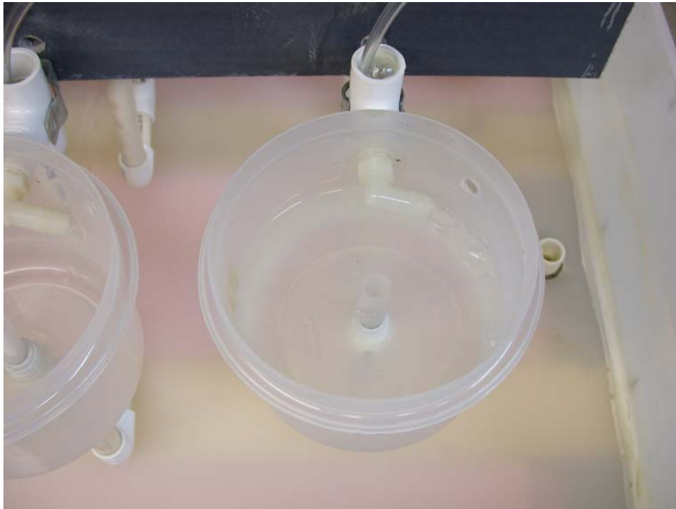
Figure I.1. Flow-through exposure chamber. Aeration in pipe creates an air lift that pumps water to the tee fitting. Exposure solution from air lift creates clockwise circular flow. Screen in center prevents test organisms from getting entrained in air lift.
