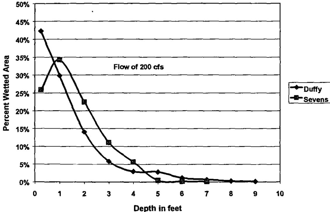
**Figure 3. Percent of wetted area for depths at a flow of 200 cfs for the Duffy and Sevens study sites.**
