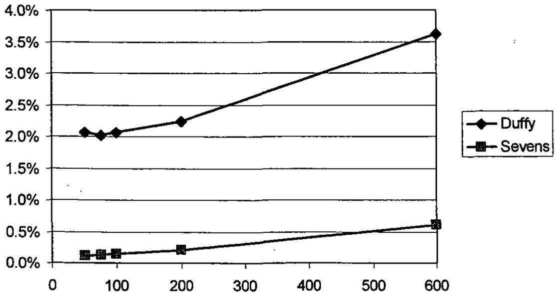
Figure A3.8. Percent of surface area at depths over 5.5 feet at Duffy and Sevens study sites at flows of 50, 100, 150, 200 and 600 cfs.
