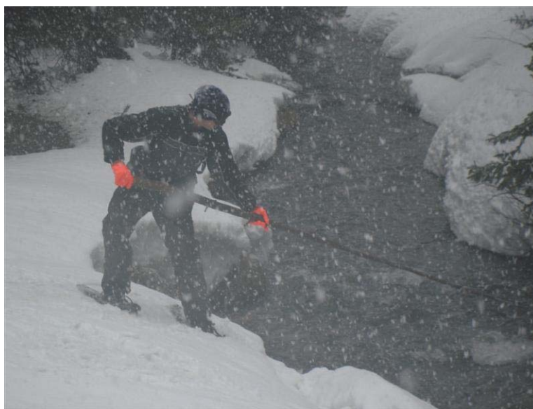
Figure 6. University of Colorado graduate research assistant Tim Dittrich samples Coal Creek from the upstream end during the April 8, 2007 synoptic sampling using snow shoes and a pole to extend the sample bottle into the stream without collapsing the snow accumulated on the north bank.
