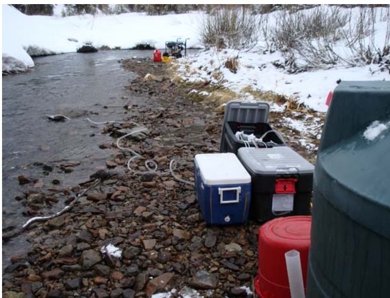
Figure 4. The injection setup at CC-3.085 for the metal loading tracer dilution test on April 8, 2007. From left to right, the tube delivering the injection solution to Coal Creek, the generator that powered the injection pump (in the background), the injection pump in the open container, and the 330 gallon injection tank (dark green, right foreground).
