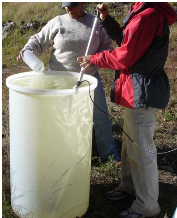
Figure 5. Lithium chloride was added to the injection solution and stirred with a paddle for 90 min until the salt was completely dissolved.
