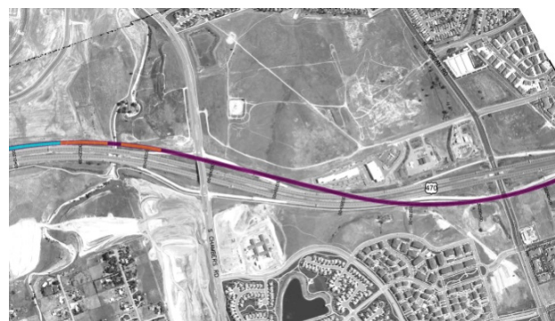
EXHIBIT 5-36: SHIFTING FROM ONE SIDE OF E-470 TO THE OTHER THROUGH CHAMBERS ROAD AND JORDAN ROAD INTERCHANGES SETS UP FLATTER ALIGNMENT TO AVOID SHARP S-CURVES AT PARKER ROAD INTERCHANGE
