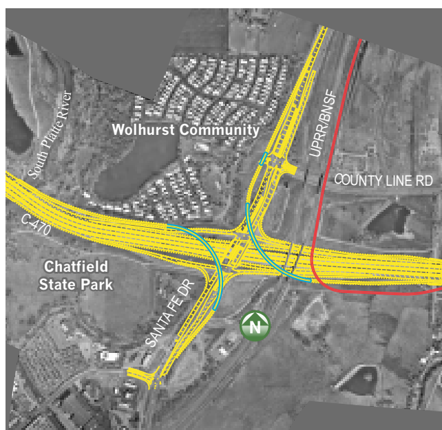
Figure 2-27 Improved Diamond Interchange with Two Flyovers Alternative
