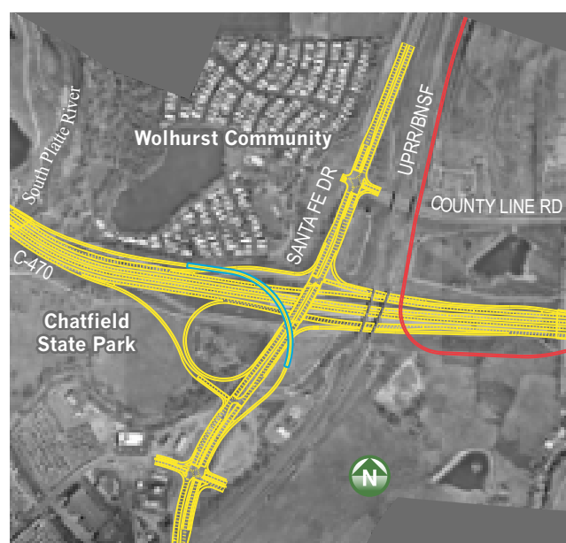
Figure 2-24 Southwest Partial Cloverleaf Interchange with One Flyover Alternative
