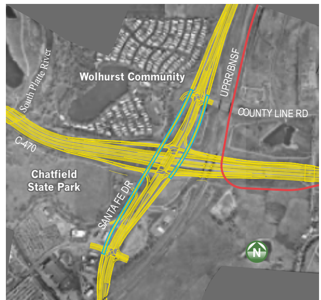
Figure 2-22 Three-Level Diamond Interchange (b) Alternative
