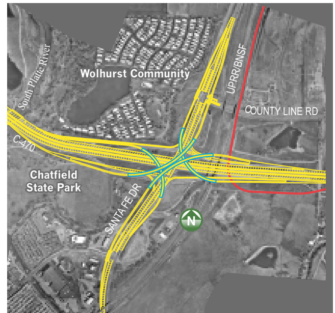
Figure 2-35 Directional Interchange Alternative
