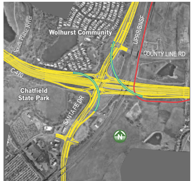
Figure 2-30 Single Point Urban Interchange with Two Flyovers Alternative
