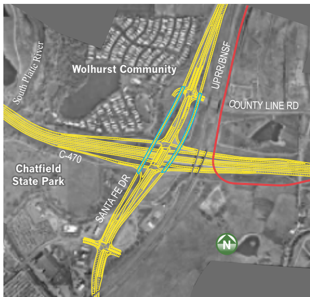
Figure 2-21 Three-Level Diamond Interchange (a) Alternative
