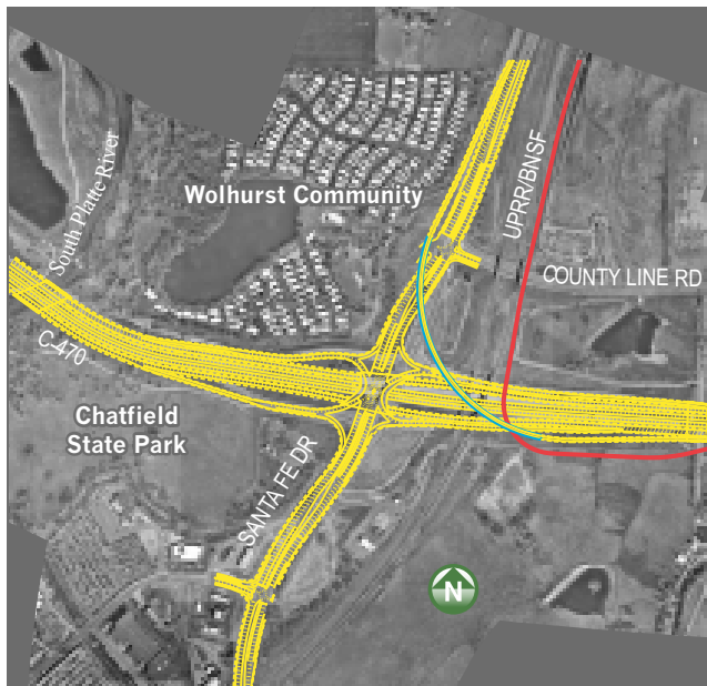
Figure 2-29 Single Point Urban Interchange with One Flyover Alternative
