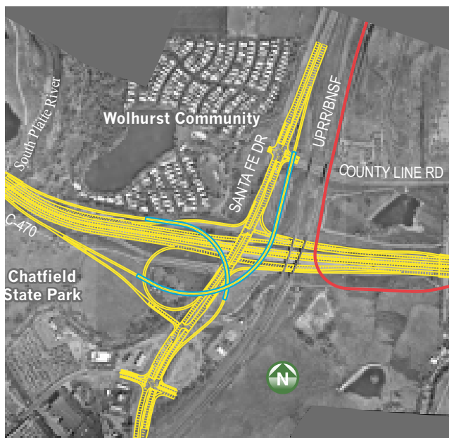
Figure 2-25 Southwest Partial Cloverleaf Interchange with Two Flyovers Alternative
