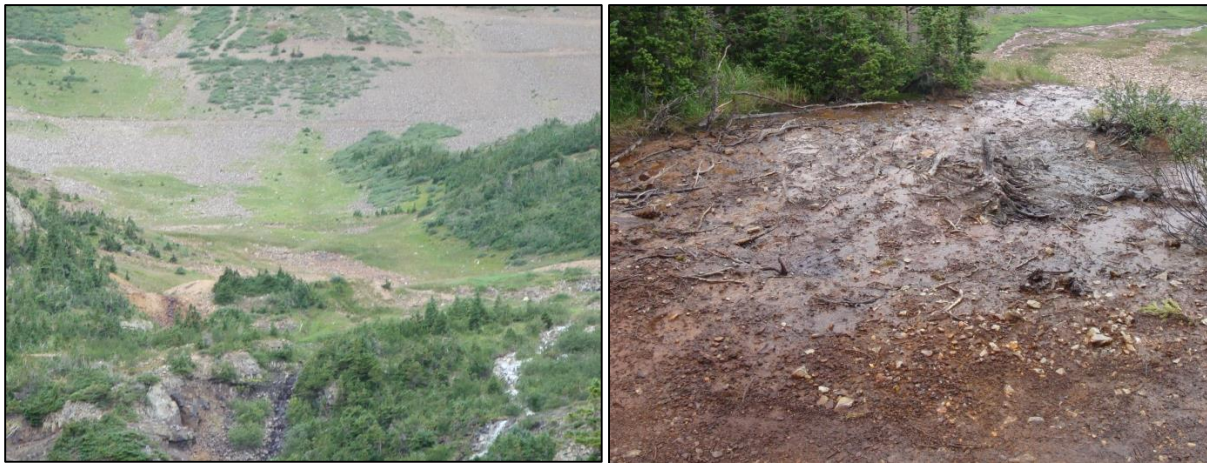
Photos 29a and b. Small abandoned mine features litter Redwell Basin and most are a part of the Daisy Mine (right Photo). Flow from the collapsed tunnel passes through waste en route to Redwell Creek (left photo).
