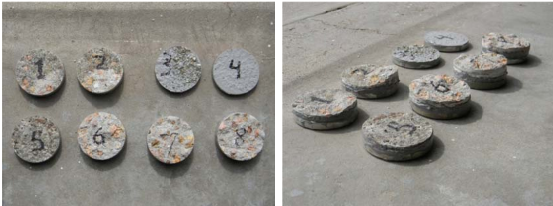
Figure 7.4.3.2: Test Cores from I-25 / I-225 Bond Testing
