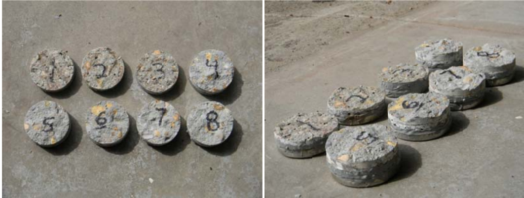
Figure 7.4.2.2: Test Cores from Parker Road / I-225 Bond Testing
