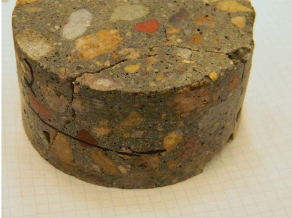
Figure 7.5.2.2: Cracked Permeability Sample R7
