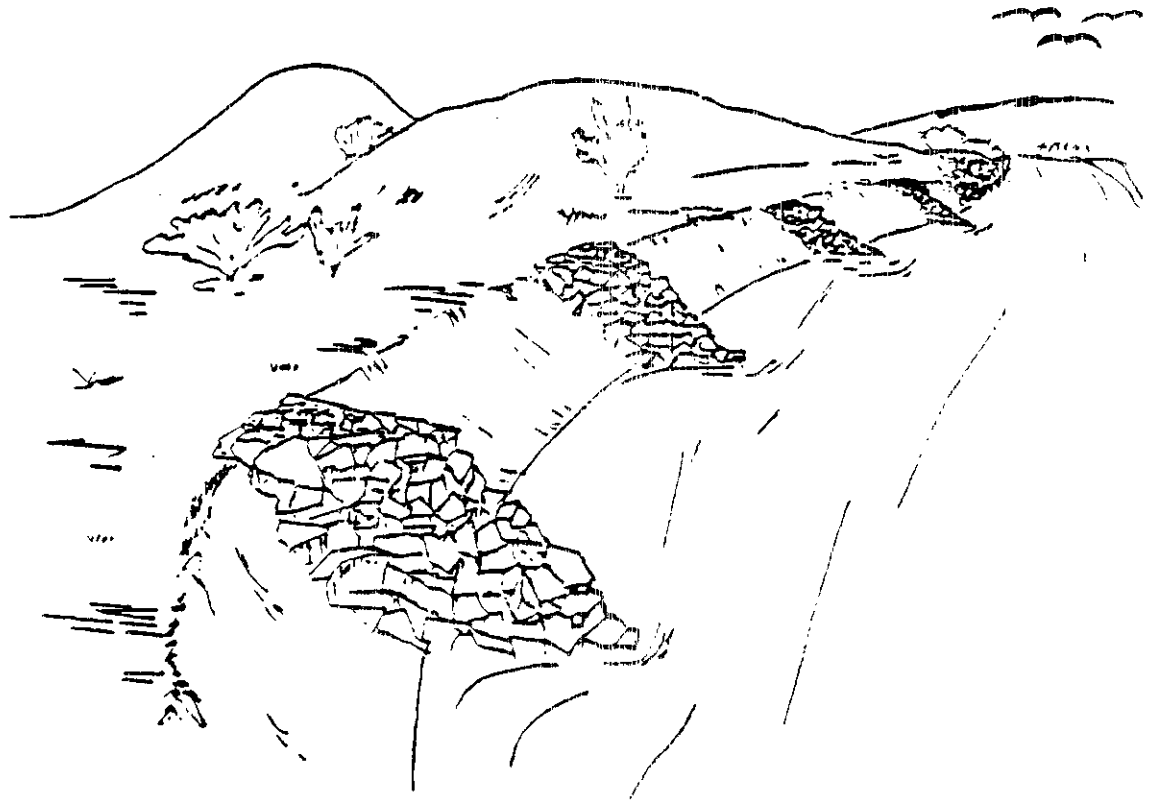
JETTY STREAMBANK EROSION CONTROL
