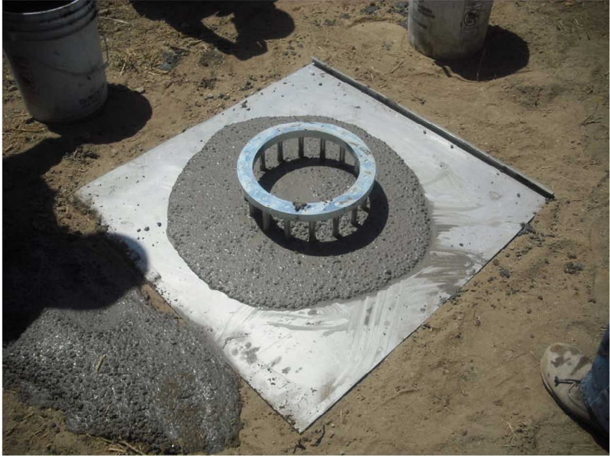
Figure 3: SCC Slump Flow Test with J-Ring
