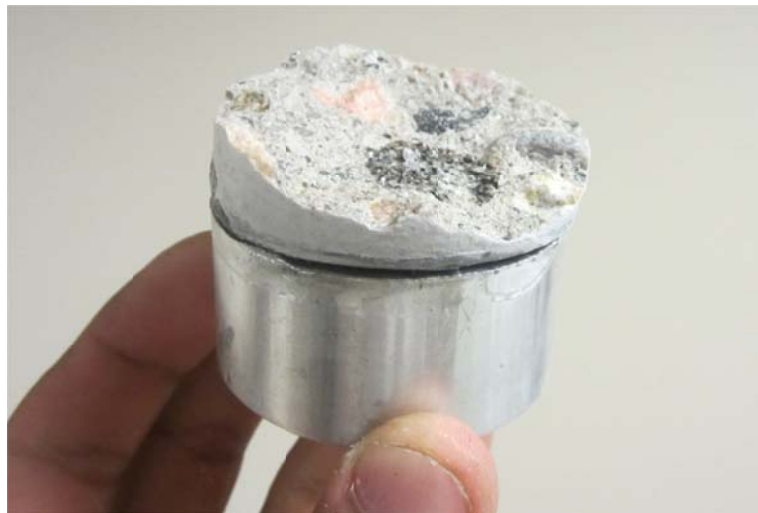
Figure 6.31. Mode G failure in dolly #20
