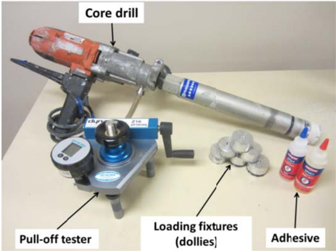
Figure 6.4. Instruments needed to conduct pull-off tests
