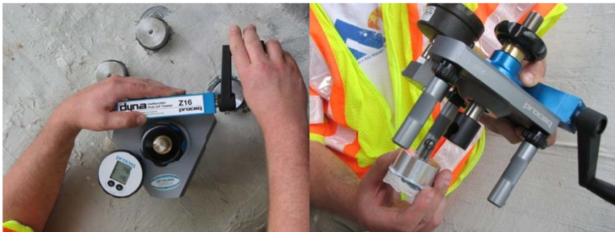
Figure 3.13. Conducting a pull-off test with the digital manometer reading and removing the tested puck from the pull-off tester
