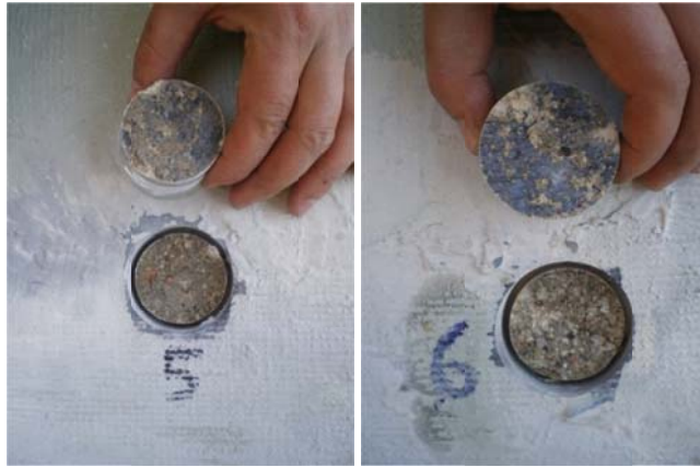
Figures B4 and B5. Test No.5, note puck slid off of center while epoxy was setting, and test No. 6
