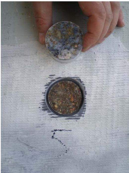
Figures B12 and B13. Test No.14, weak bond strength, and test No.15, weak bond strength
