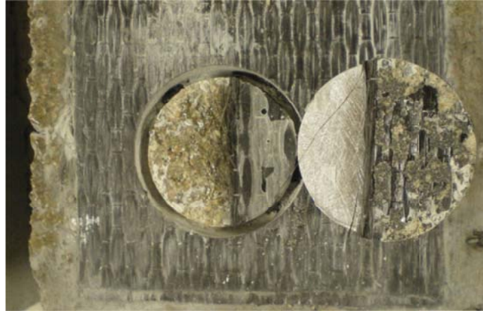
Figure 6.28. Combined Mode A and Mode F failure
