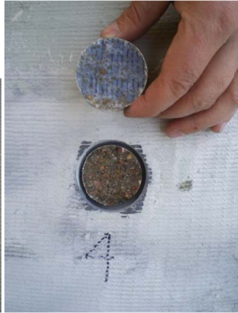
Figures B10 and B11. Test No.12, weak bond strength, and test No.13, weak bond strength
