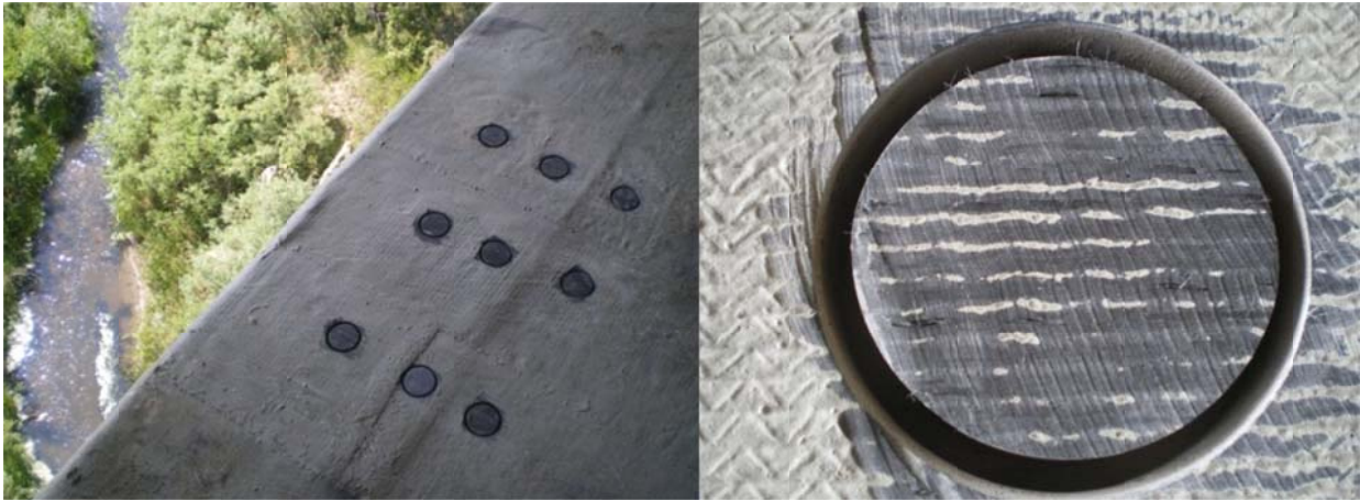
Figure 3.9. Prepared areas for the adhesion of aluminum pucks for pull-off tests and a close-up of a prepared surface
