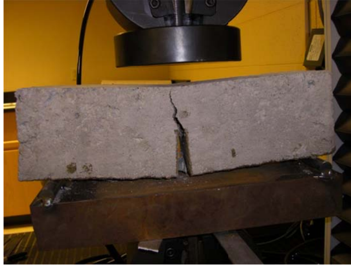
Figure 6.22. Beam following crack failure
