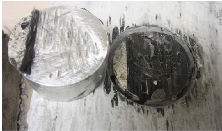
Figure 6.33. Combined Mode A and Mode F failure in dolly #42
