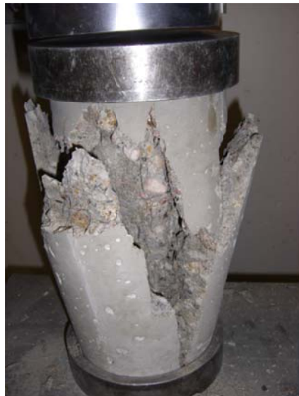
Figure 6.17. Characteristic failure for compression tests
