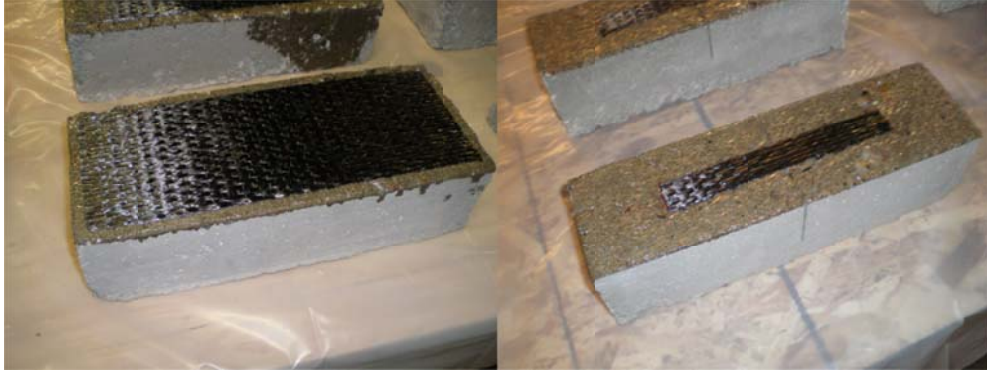
Figure 6.11. Concrete specimens reinforced with CFRP for pull-off (left) and flexural (right) tests
