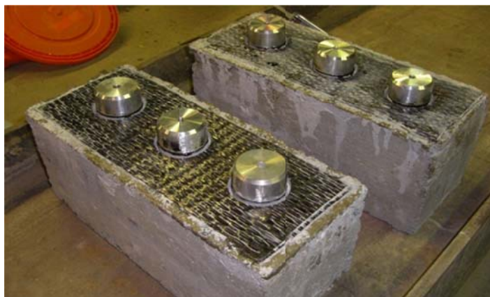
Figure 6.13. Concrete specimens following adhesion of dollies
