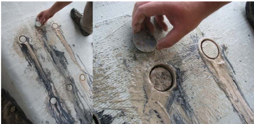
Figure 3.6. The core drilling location that failed due to torsional stresses during the core drilling process, bay 1NW
