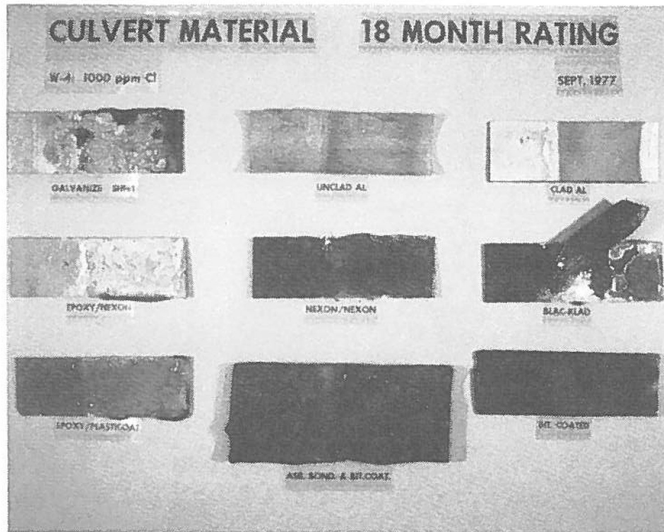
Photograph No. 15 Metal samples after 18 months in a harsh water environment
