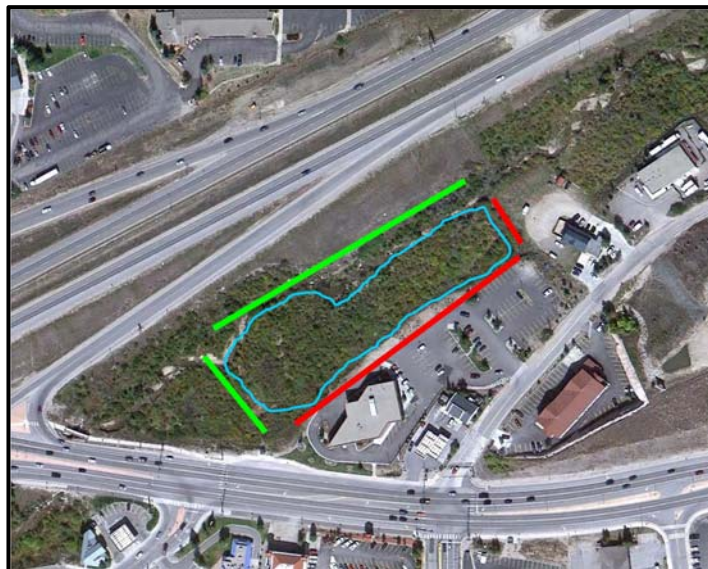
Figure 33. A FACWet test site on Straight Cr. in Summit County, along the I-70 corridor. The blue outlined polygon is the AA. Green lines indicate where buffer land cover exceeds 5m in width. Red lines mark where no buffer exists. Fifty-two percent of this test site had buffer, placing it at the bottom of the functioning category (~0.72).
