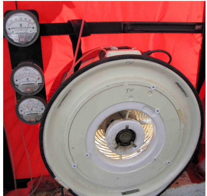
Figure 3-19. Close up with meters. Low flow calibration plate used because structure is quite tight.
