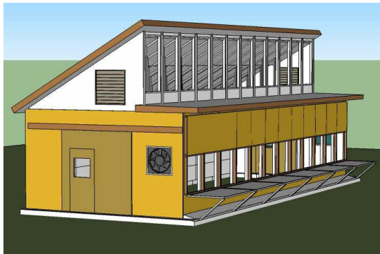
Figure 3-3. SW elevation showing fan, louver, door within a door (larger for tractor, smaller for people), fixed light shelf on roof, variable light shelves on south side, 12 roof windows and 12 south wall windows.
