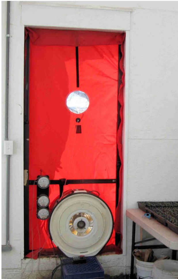
Figure 3-18. Blower door set up, east door.
