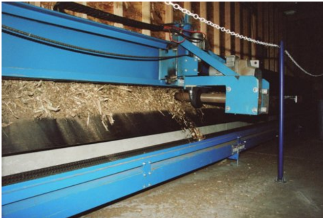
Figure 2.3 Storage Bin Auger
