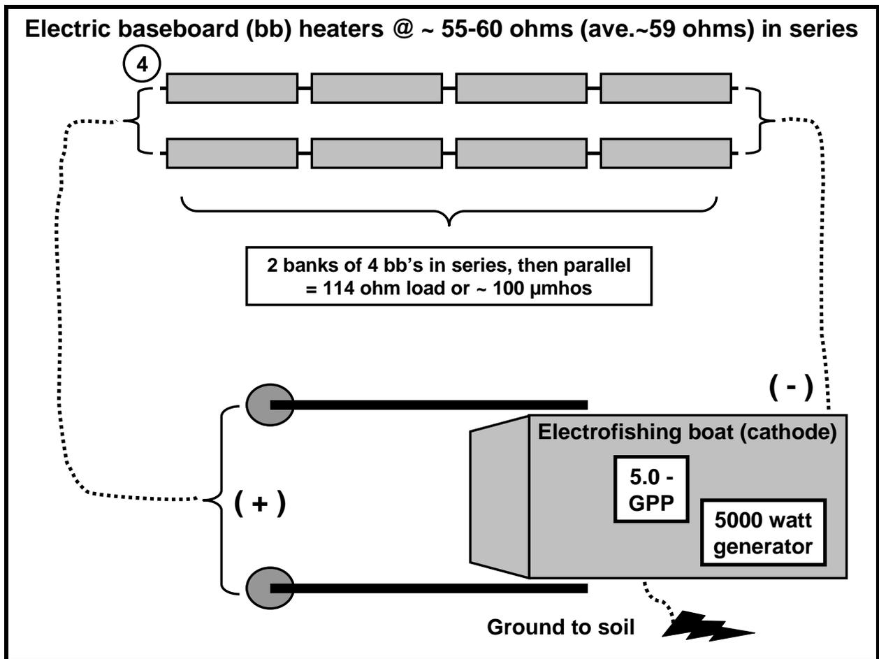
**Figure 6.** Diagram of set-up for subjecting a Smith-Root Model 5.0-GPP electrofisher to a fourth level of electrical resistance of 114 ohms using two arrays of four baseboard heaters in series, then parallel, to simulate a water conductivity of 100  $\mu$ hos.
