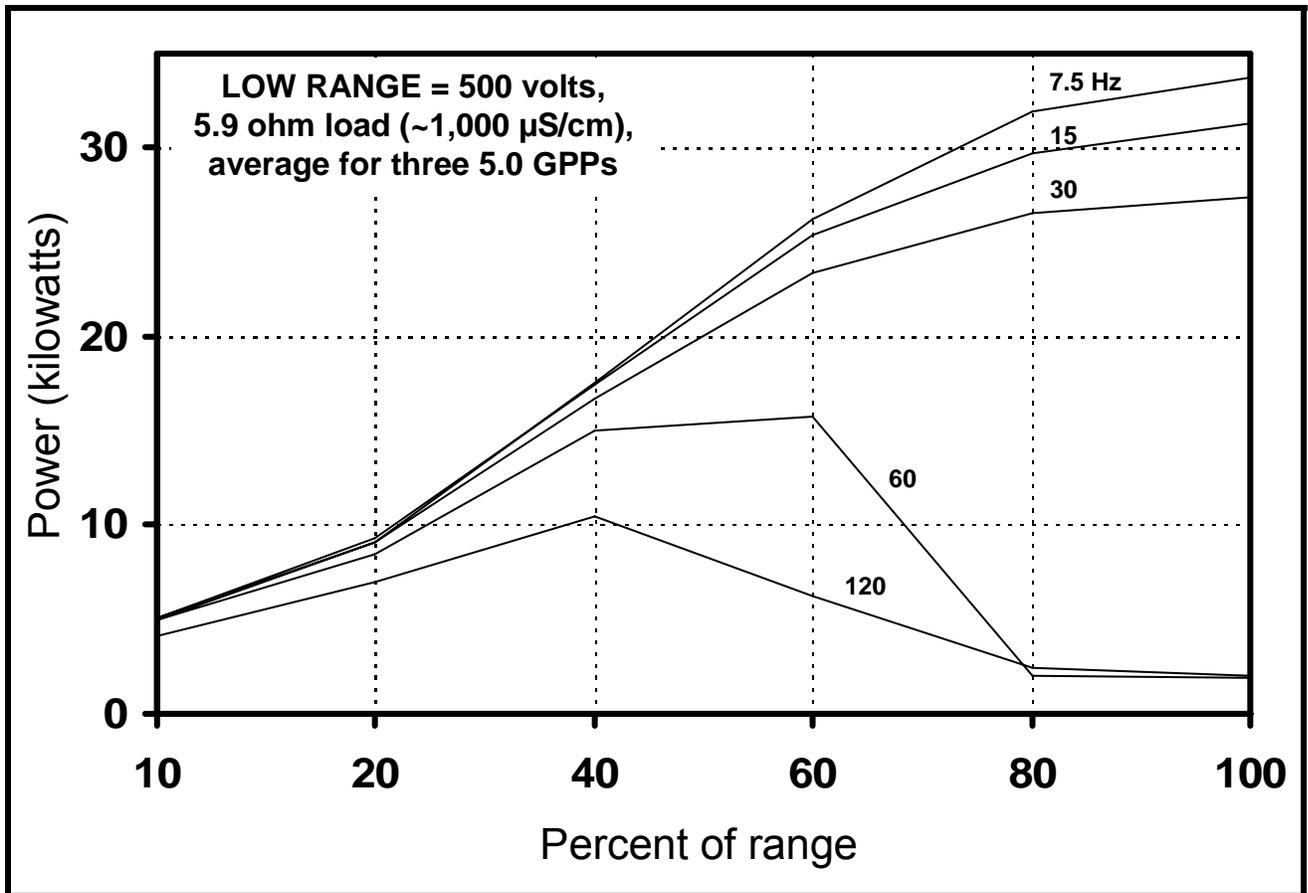
**Figure 11.** Power output for Smith-Root Model 5.0 GPP electrofisher, averaged for three units, operating at the LOW RANGE 500 volt setting in the DC mode (Figure 1). Electrofishers were subjected to an electrical load of 5.9 ohms simulating an approximate water conductivity of 1,000  $\mu$ S/cm, as illustrated in Figure 3, and operated at percent of range settings of 10, 20, 40, 60, 80 and 100 at pulse per second settings of 7.5, 15, 30, 60 and 120 Hz.
