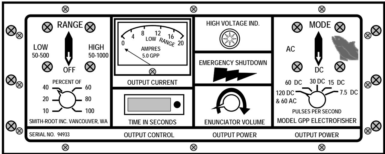
**Figure 7.** Control panel of Smith-Root Model 5.0-GPP electrofisher.
