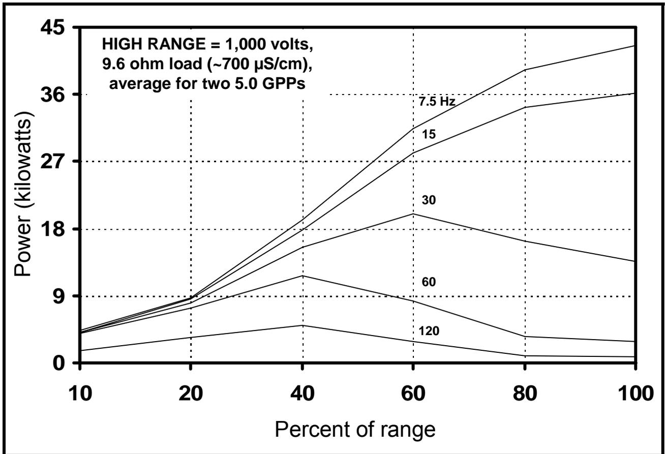
**Figure 14.** Power output for Smith-Root Model 5.0 GPP electrofisher, averaged for two units, operating at the HIGH RANGE 1,000 volt setting in the DC mode (Figure 1). Electrofishers were subjected to an electrical load of 9.6 ohms simulating an approximate water conductivity of 700  $\mu$ S/cm, as illustrated in Figure 3, and operated at percent of range settings of 10, 20, 40, 60, 80 and 100 at pulse per second settings of 7.5, 15, 30, 60 and 120 Hz.
