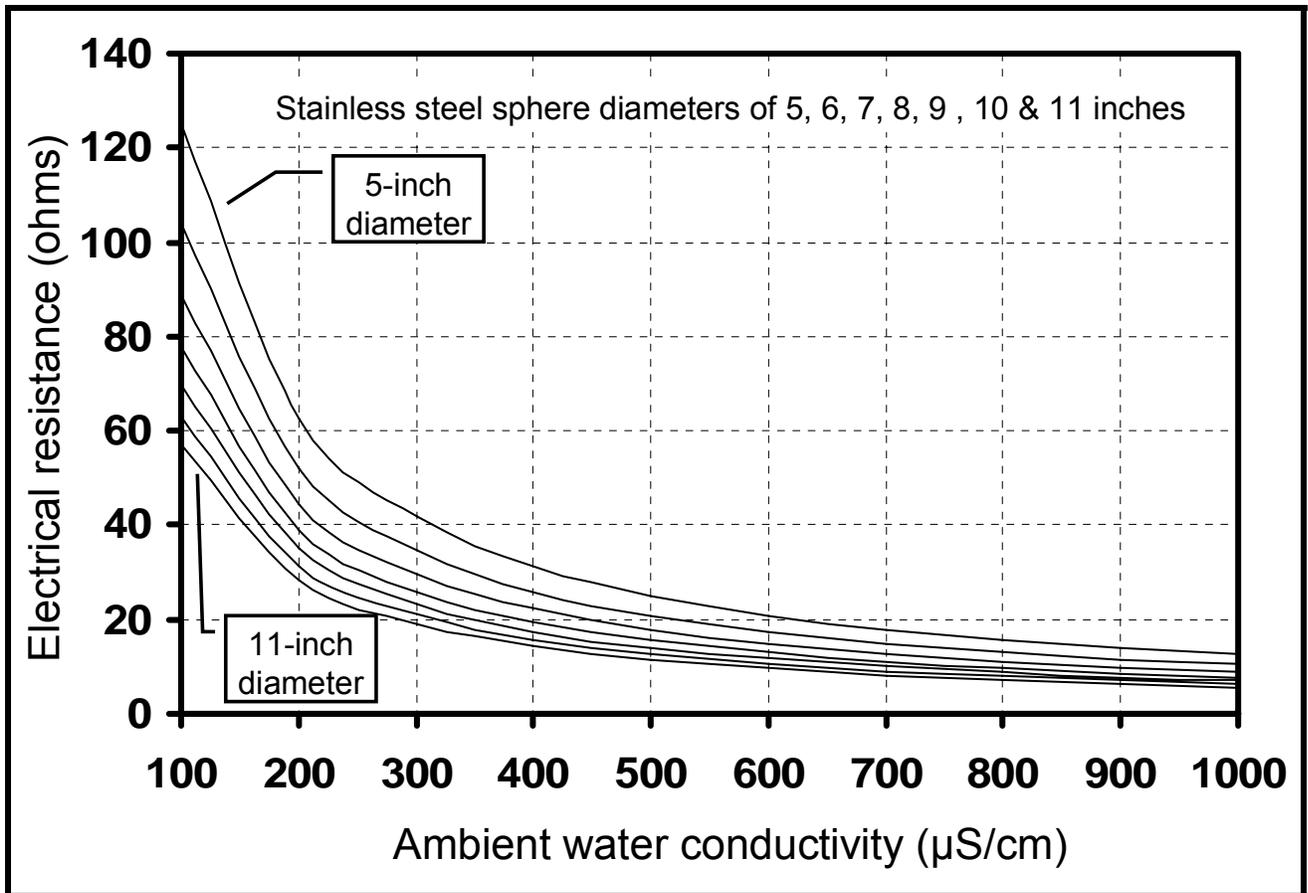
**Figure 4.** Theoretical electrical resistance of stainless steel spheres of 5, 6, 7, 8, 9, 10, and 11 inches in diameter at water conductivities ranging from 100 to 1000  $\mu\text{S}/\text{cm}$ .
