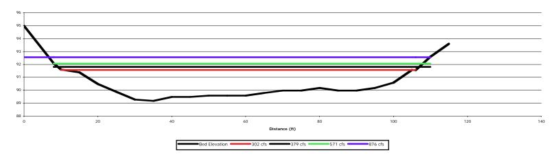
Roaring Fork at the Tree Farm, Cross Section 2 Bed and water surface elevation
