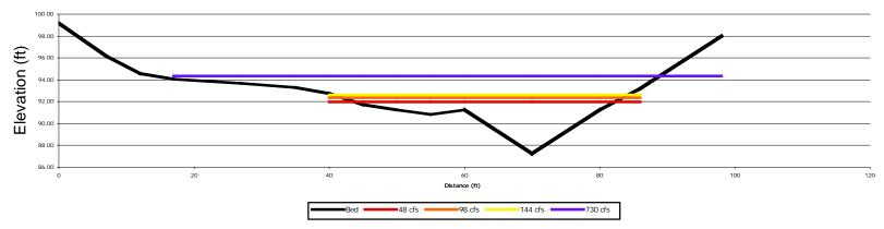
Figure 3-44. Comparison of Water Surface Elevations for High-Risk Flows and Average August-September Flows for RFR-TF Cross Section 5
