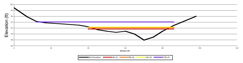
Figure 3-43. Comparison of Water Surface Elevations for High-Risk Flows and Average August-September Flows for RFR-TF Cross Section 4
