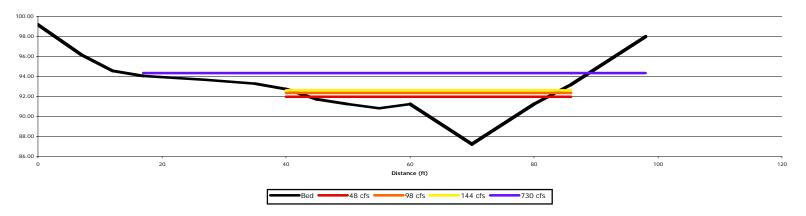
Water Surface elevation versus discharge, Roaring Fork Cross Section 5
