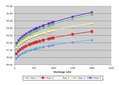
Figure 3-38. Stage Discharge Function for Site RFR-TF
