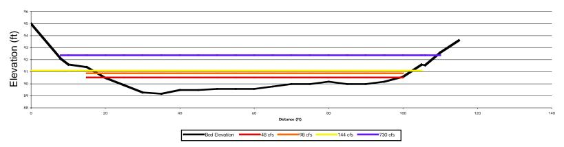
Figure 3-41. Comparison of Water Surface Elevations for High-Risk Flows and Average August-September Flows for RFR-TF Cross Section 2
