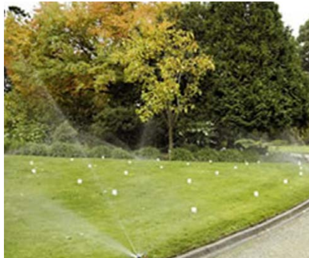
Placement of catch cans for irrigation efficiency audit. Photo Source: Kenneth Solomon
