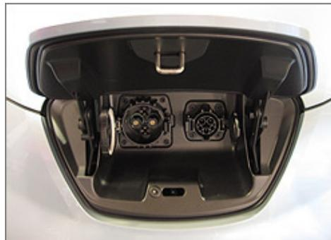
**Figure 1:** The standard receptacle (right) can receive charge from level 1 or level 2 equipment. The DC fast charge receptacle (left) uses a different type of connector. Photo courtesy of National Renewable Energy Laboratory.
