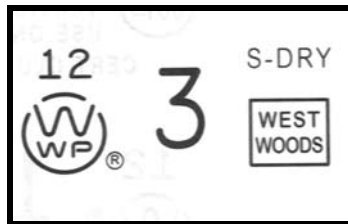
Figure 1. Grade stamp for No.3 lumber made of the species combination western woods.
