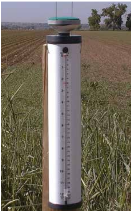
An atmometer estimates crop water use to help better schedule irrigation.
