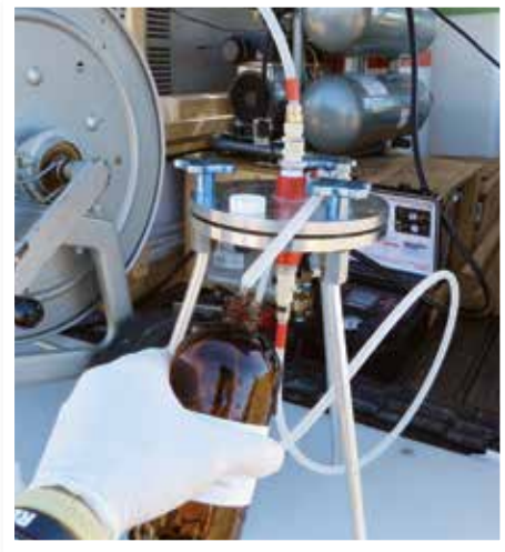
Program technicians utilize standardized and approved equipment and techniques for collection of groundwater samples.
