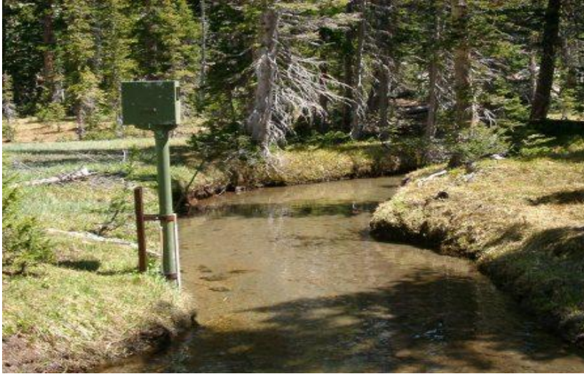
Figure 26: Stream Gauge on Andrews Creek, CO;
