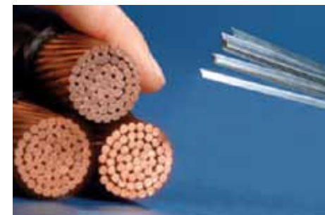
Figure 97: The few ultrathin high-temperature superconducting wires on the right carry as much power as all the copper shown on the left. Source: AMSC 212
