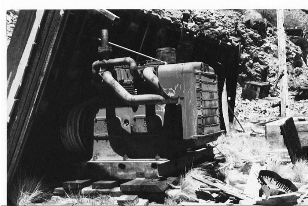
Figure E 5.2.35. The V-cylinder compressor, similar to a large engine, became one of the most popular compressor types after the 1930s. Note the foundation. Source: Twitty, 2002:274.
