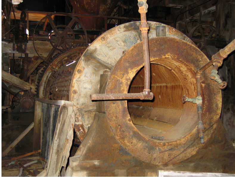
Figure F 6.6. Rod mills such as the one at the Cardinal Mill became popular for fine grinding by the 1910s. As the entire cylinder slowly rotated, tumbling steel rods in the chamber ground screened ore into a slurry. A hatch covered the opening. Source: Carol Beam.
