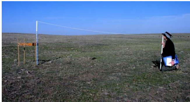
Georgia Doyle estimating vegetation height using the Robel pole visual obstruction method.
