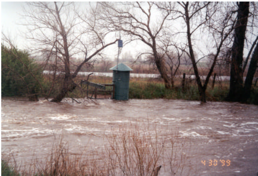
USGS gaging station on Poudre River near BSD facility. Station was rendered inoperable by flood flows.
