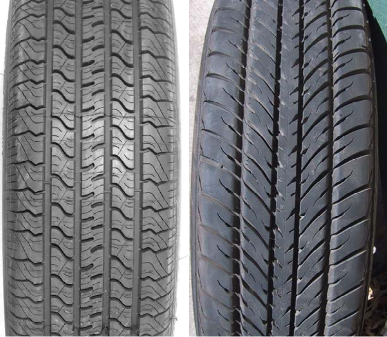
Figure A.2. Test tires – ASTM F 2493 SRTT and Goodyear Aquatred III.
