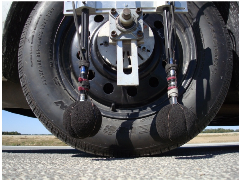
Figure A.1. OBSI measurement bracket configuration.
