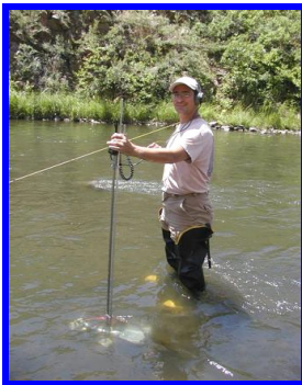
Water Commissioner measuring flow of water
