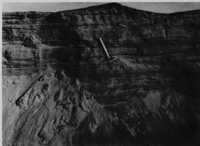
Figure 5. Fountain Sand and Gravel Company hydraulic sands in El Paso County. This deposit supplies the petroleum industry in the United States and Canada with coarse-grained quartz sands that are used to increase the recovery of oil. The pit is located 1 mile east of the south entrance of the U. S. Air Force Academy. Photograph by P. C. Wicklein.
