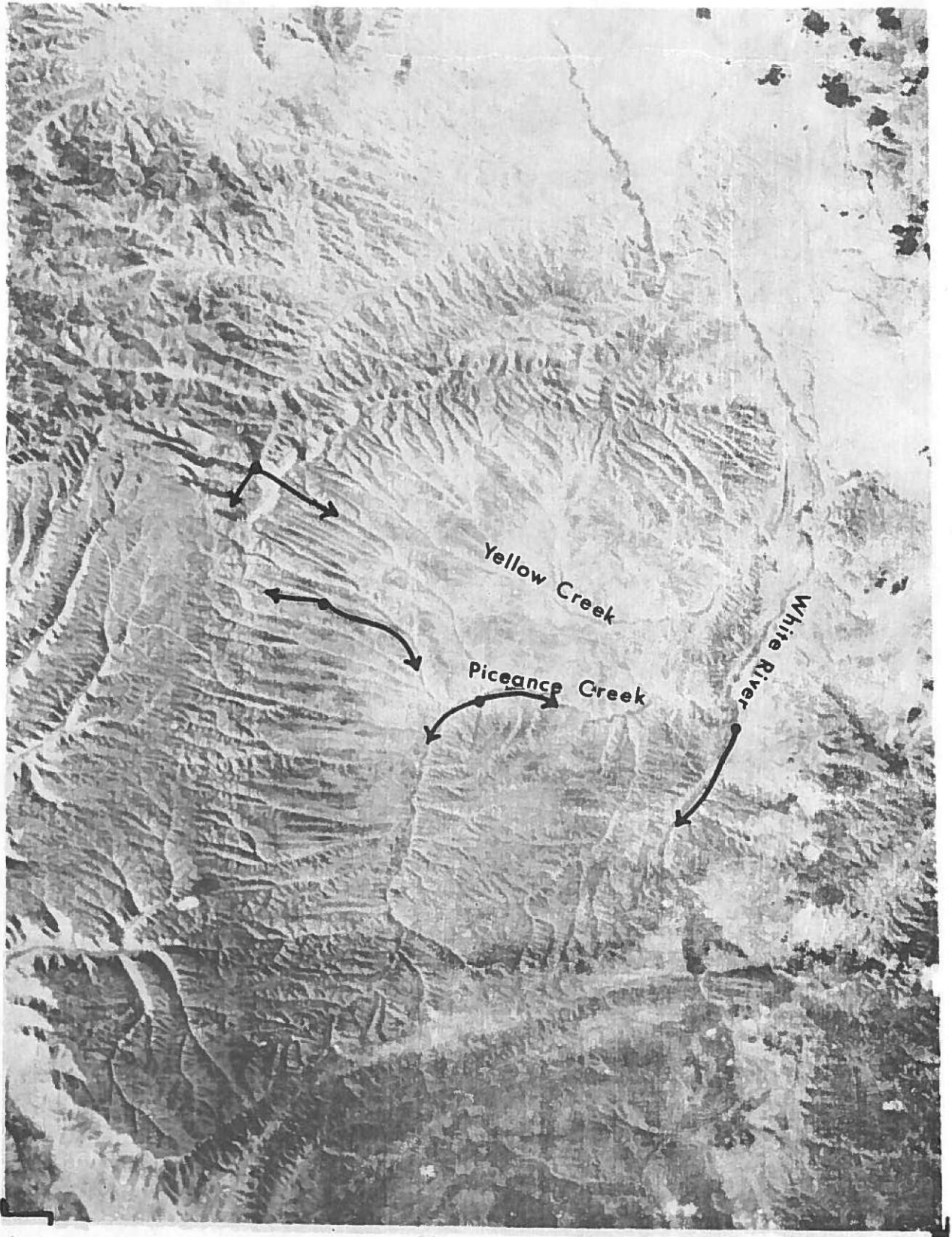
Figure 7. Wind Flow Patterns for the Piceance Creek Basin. March, April - 1400, 1500, 1600 HRS.
