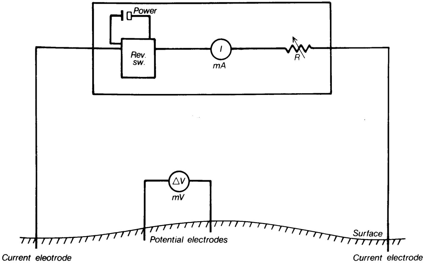
Figure 18. Schematic diagram for resistivity (from J. Combs, 1980).
