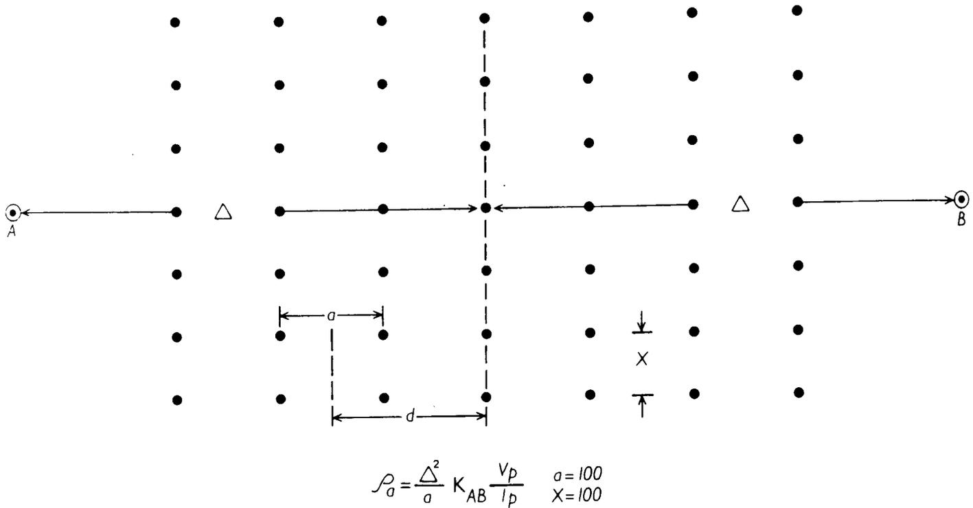
Figure 11. Plan view of the gradient array, or AB rectangle array. The rectangular area between distant, fixed current electrodes is traversed by a pair of potential measuring electrodes. Although the array factor  $K_{AB}$  is near unity, it is a variable.
