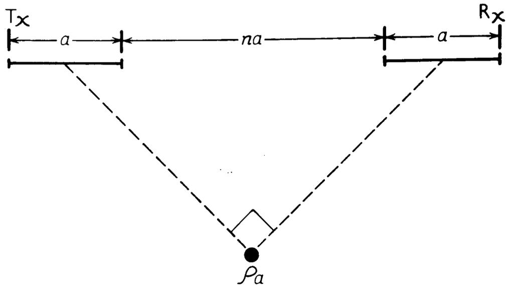
Figure 22. Data plotting scheme for dipole-dipole array (from J. Combs, 1980).
