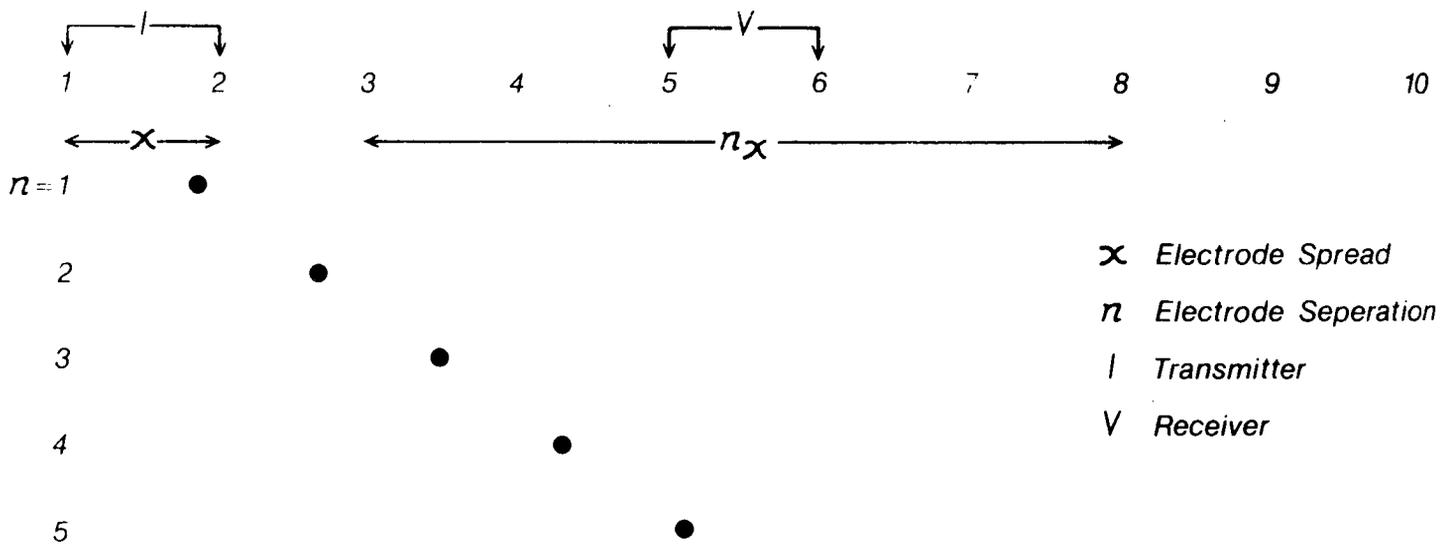
Figure 23. Typical dipole-dipole array (from J. Combs, 1980).
