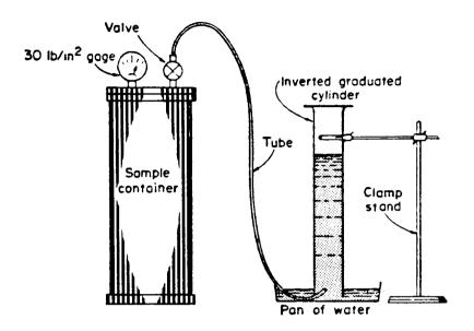
Figure 23. Methane desorption equipment (after McCulloch and others, 1975, p. 4).
