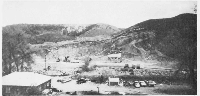
Figure 8. Andesite Rock Company quarry on South St. Vrain Creek southeast of Lyons. This rhyolite sill intrudes east (left)-dipping sandstones and dark shales of the Pennsylvanian Fountain Formation. Photo by James Soule, Colorado Geological Survey.
