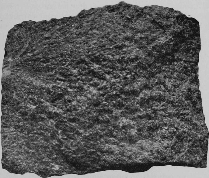
Fig. 2. Monzonite porphyry, from the west side of the Alamosa River, opposite the Gilmore meadow. Natural size. See page 42.
