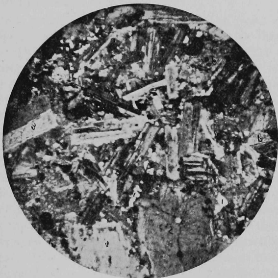
Fig. 1. Photomicrograph of monzonite, from the west side of the Alamosa River below Bitter Creek. \times 15 . Polarized light. The figure shows orthoclase (2), plagioclase (3), quartz (1), augite (6), and magnetite (black). See page 42.
