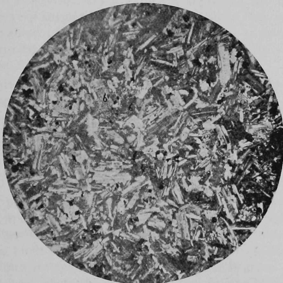
Fig. 2. Photomicrograph of biotite-augite diorite, from Wightman's Fork. The same rock as shown in Figure 1. \times 15 . Polarized light. The figure shows light-colored plagioclase strips, biotite (4), augite (6), and magnetite (black). See page 45.
