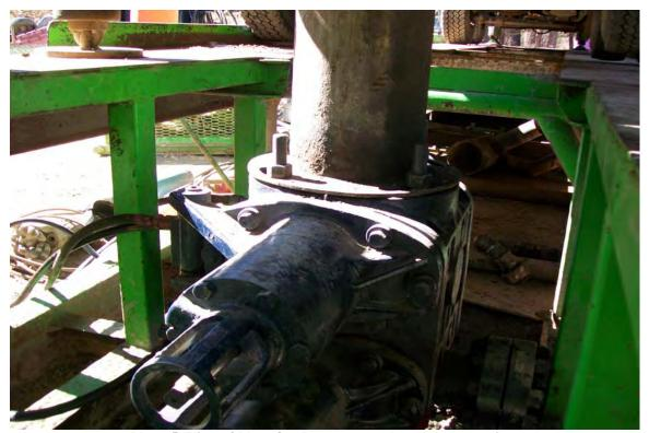
Photo 5: View of Blow-Out Preventer on the conductor casing.
