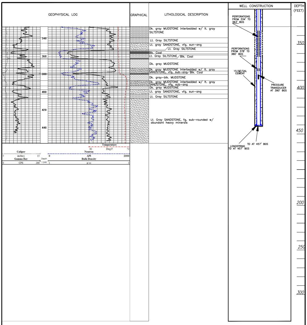
BORE HOLE: 12 1/4" TO 44' BGS CONDUCTOR CASING: 9 5/8" 36# STEEL TO 43' BGS CEMENT: 15.5#/GALLON TO SURFACE BORE HOLE: 8 3/4" TO 282' BGS SURFACE CASING: 7" 20# STEEL TO 271' BGS CEMENT: 15.5#/GALLON TO SURFACE BORE HOLE: 6 1/4" TO 457' LONG STRING: 4 1/2" 10.5# STEEL TO 457' BGS CEMENT: 15.5#/GALLON TO SURFACE PERFORATIONS: 174-190, 220-226, 276-291, 334-363,
