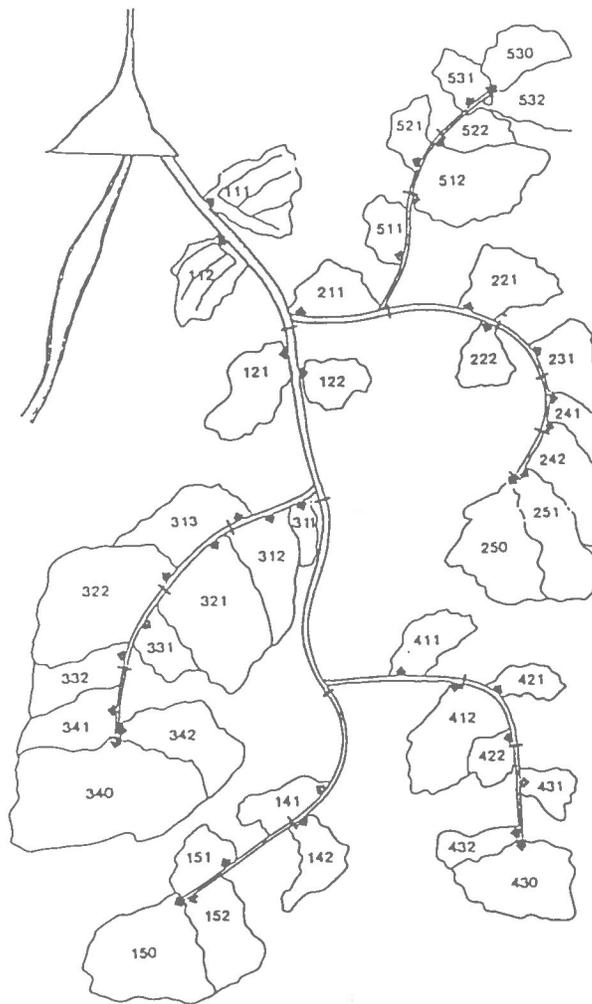
Figure 1. Branching Canal Network Showing Command areas
