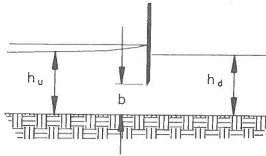
Figure 3. Flow through Orifice Type Structures
