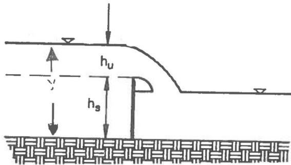
Figure 2. Flow through an Overflow Structure
