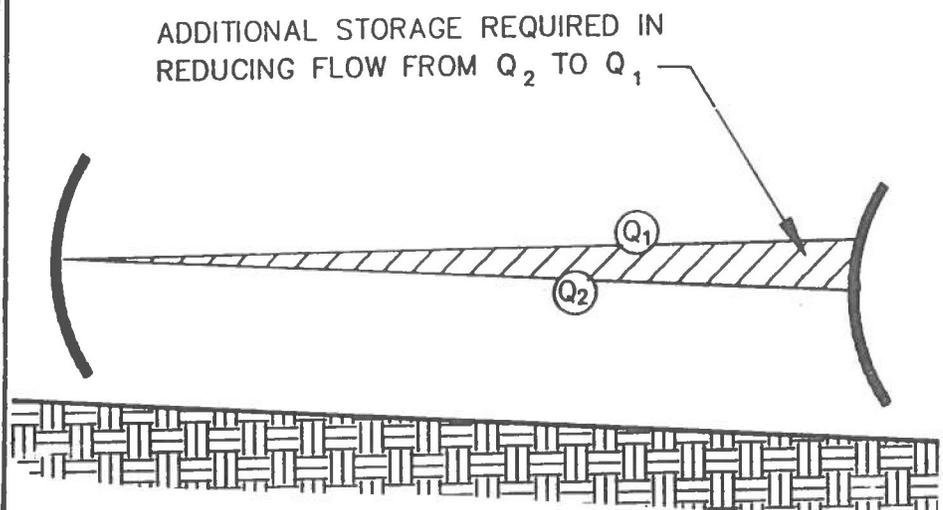
Figure 8. Water surface profile for downstream control
