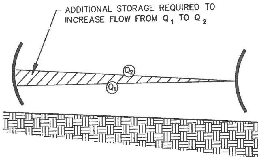
Figure 7. Water surface profile for upstream control
