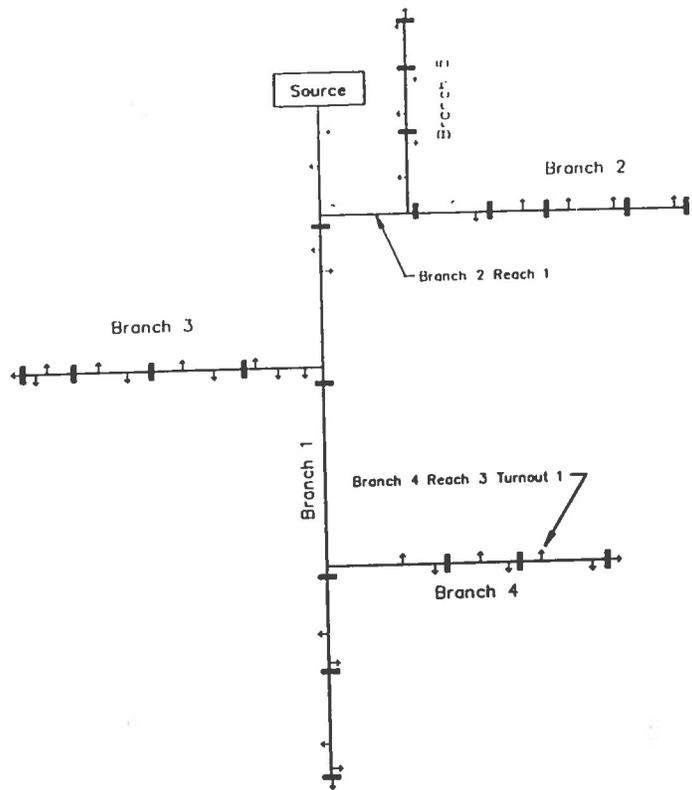
Figure 10. Schematic Representation of a Branching Canal Network
